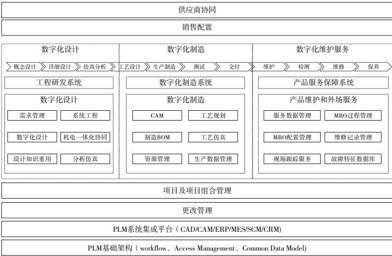
Fig. 2 Implementation of digital coverage of enterprise main business processes based on PLM software
